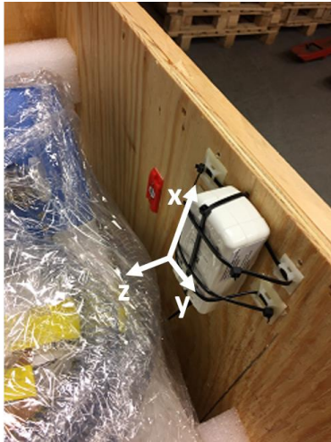
Tracking device mounted in a wooden transportation crate.
